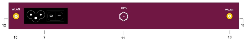
Fig. 3: bintec RS353j-4G rear panel
