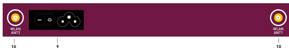
Fig. 8: bintec RS123w , bintec RS353aw rear panel
