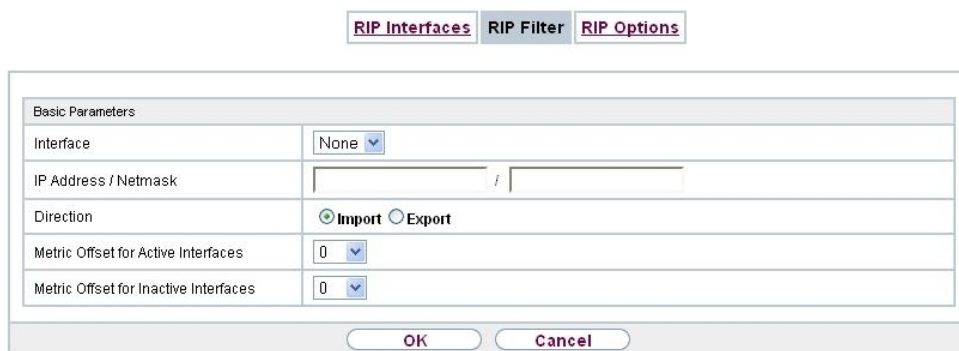
Fig. 117: Routing Protocols->RIP->RIP Filter->New
