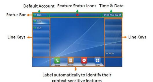
For SIP-T46S/T46G IP phone, the page icons appear only when you assign functionality to line key located in line key 11-27, refer to DSS Keys for more information. The wallpaper can be customized, refer to Changing Wallpaper on the Idle Screen for more information. The Idle screen on SIP-T46S/T46G IP phone is shown as below:
