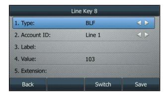
The Line Key screen on the SIP-T40G/T40P IP phone is shown as below:
