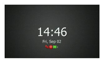
For the SIP-T48S/T48G/T46S/T46G IP phone, you can upload custom pictures to set up a screen saver of your picture, configure the screen saver type and screen saver display clock. For all IP phones, you can also configure the screen saver wait time and configure the phone whether to display custom XML items (for example, notifications or company logo) on the screen saver or not. The custom XML items are preset by your system administrator.
