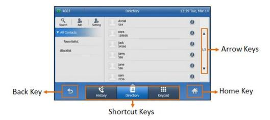
On SIP-T46S/T46G/T42S/T42G/T41S/T41P/T40G/T40P IP phone, you can press the navigation key to switch among the groups. The Directory screen on SIP-T46S/T46G IP phone is shown as below:
