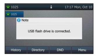
If you insert a USB flash drive to the IP phone during a call, a message will pop up to tell you how much time is available for recording. For more information on the available recording time, refer to Viewing the Storage Space.
