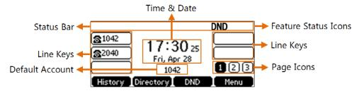
The Idle screen on SIP-T40G/T40P IP phone is shown as below:
