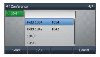
On the SIP-T48S/T48G IP phone, tap the desired hold call from the left sidebar.
